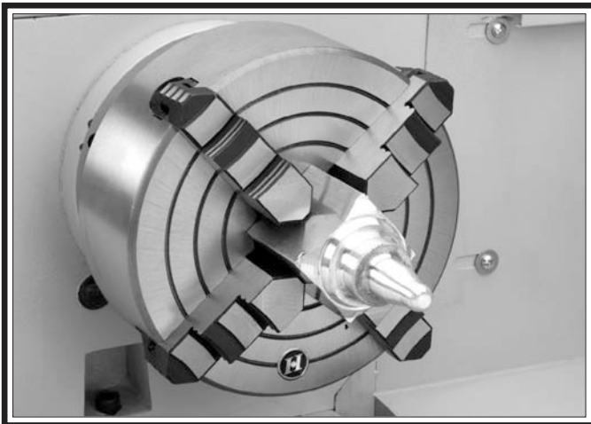
Figure 44. Example photo of non-cylindrical workpiece correctly mounted on the 4-jaw chuck.
